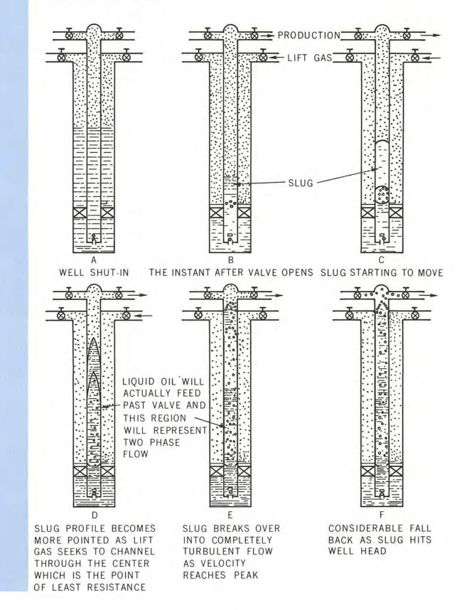
Figure 46 is a schematic diagram of intermittent gas lift operation. The gas injected into the tubing string lifts liquids to the surface by (1) reduction of fluid gradients, (2) expansion of injected gas, and (3) displacement of fluid by compressed gas.
