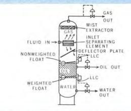
VERTICAL THREE-PHASE OIL-GAS-WATER SEPARATOR
