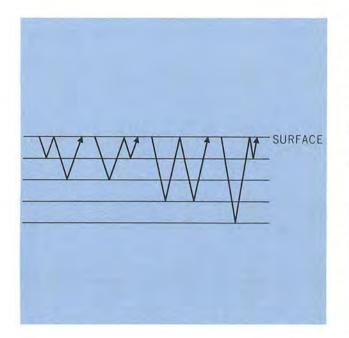
FIGURE **7** Examples of Internal Multiple Reflection Paths
