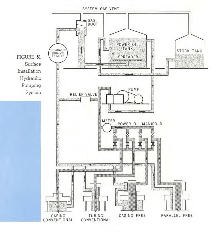
In the closed power oil system, exhausted power oil is returned to the surface and back to the power oil tank through a separate flow passage rather than being commingled with the produced well fluids.
