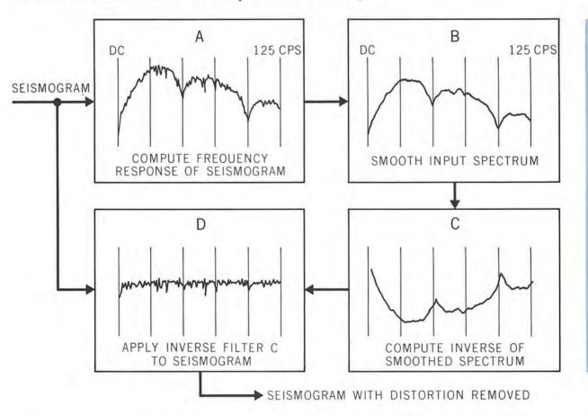
FIGURE 12. Distortion Removal by Inverse Filtering
