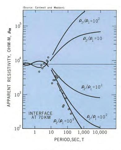
Figure 23 shows an application of the magnetotelluric method to actual field measurements in Massachusetts where the interpretation is in terms of the simple theoretical model of Figure 22.
