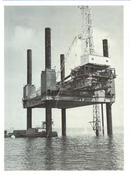
FIGURE **95** Jack-Up, Workover Rig at Caisson Supported Well
