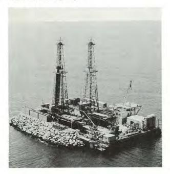
FIGURE 77 500-Ton Derrick Barge. Barge is 100' X 400'. Pipe Line-Laying Ramp and Equipment in Foreground
