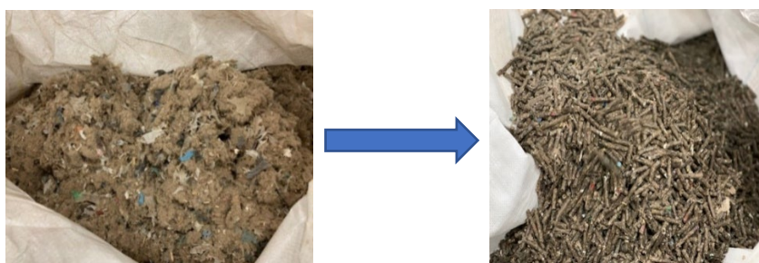
Figure 25. Pelletization of shredded MSW produces a densified material with reduced physical and mechanical variability.
