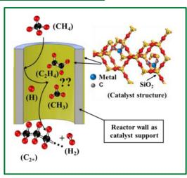
Design for isolated metal atoms in silica built into a catalytic wall reactor as part of an NETL collaboration with the University of Maryland
