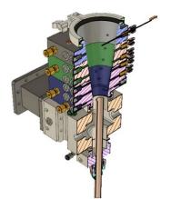
Design concept for a modular fluidized bed component as part of a microwave plasma reactor development collaboration between NETL and West Virginia University
