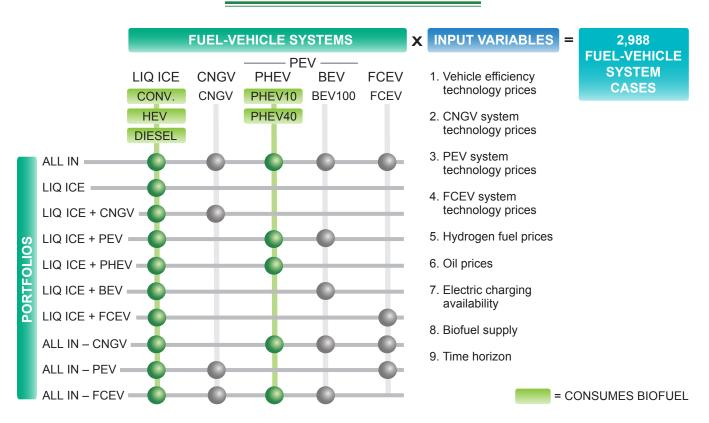
Figure 2-3. Fuel-Vehicle System Combinations Used in Analysis
