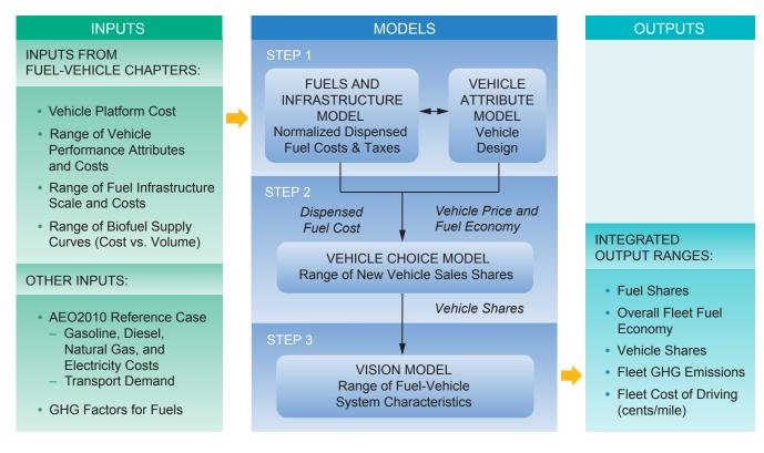
Figure 2-2. Light-Duty Analysis Process
