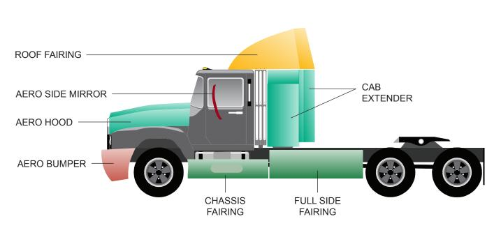
Figure 10-7. Typical Passive Aerodynamic Measures Implemented on Modern-Era Truck Tractors
