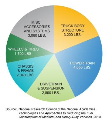
*Figure 10-8. Typical Weight Contribution of Major Subsystems of a Class 8 Line-Haul Truck*
