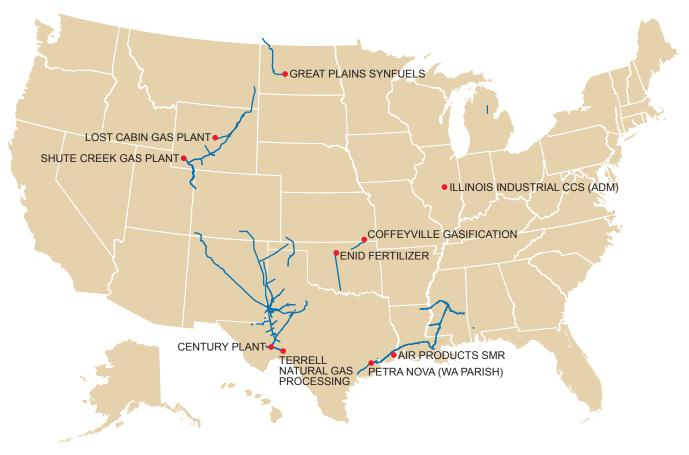
Figure 6-2. Schematic Map of CO<sub>2</sub> Pipelines in the United States
