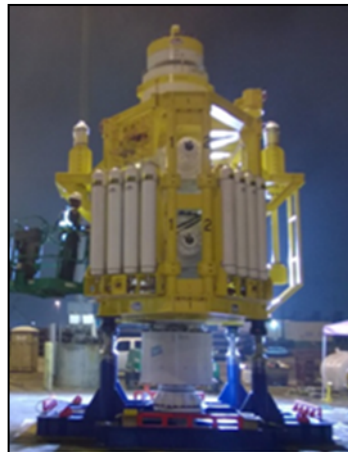
Subsea Isolation Device
