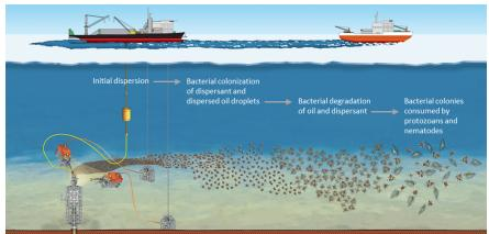
Figure 3. Subsea dispersant injection as it might be applied in ice.
