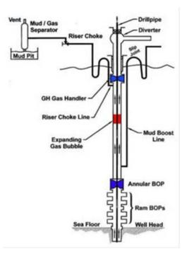
Figure 7. Well Control Equipment for a Subsea Well (note gas handler is optional)
