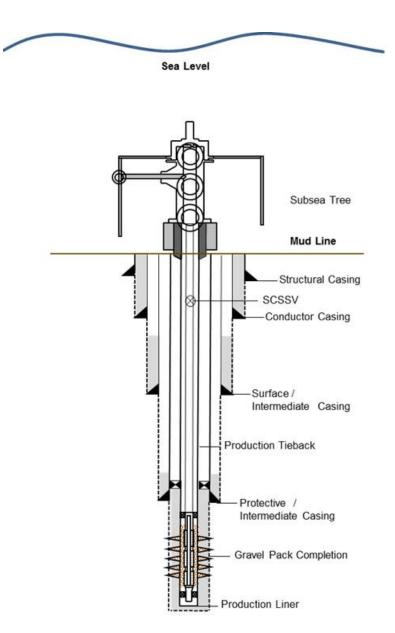
Figure 5. Schematic of a Subsea Drill Well - Completion/Production Phase
