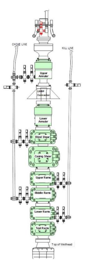
Figure 6b. Typical Subsea Blowout Preventer Stack (multiple redundancy)
