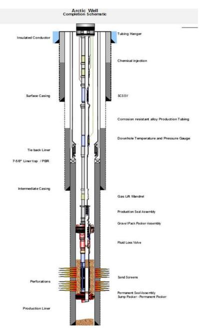
Figure 15. Example of an arctic well completion
