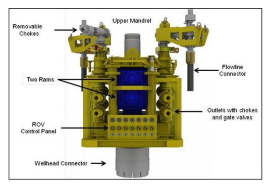
Figure 11. Example of a Dual Ram Capping Stack
