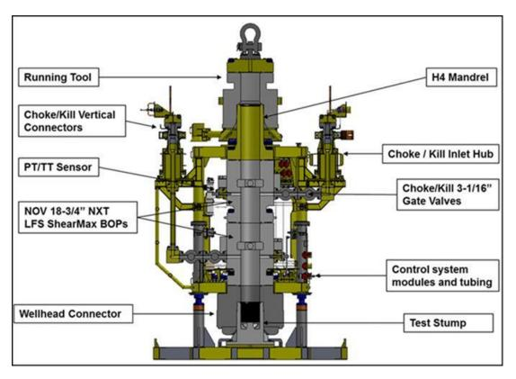
Figure 13. Internal View of a Subsea Shut-in Device
