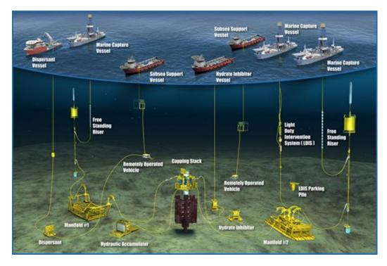
Figure 14. Illustration of a Well Containment System Utilizing Multiple Surface Processing Vessels
