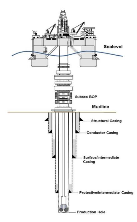
Figure 3. Schematic of a Subsea Drill Well – Drilling Phase
