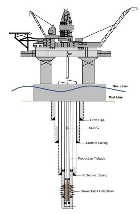
Figure 4. Schematic of a Surface Drill Well – Completion/Production Phase
