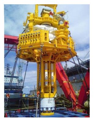
Figure 9. Capping Stack, Shell Arctic Capping Stack
