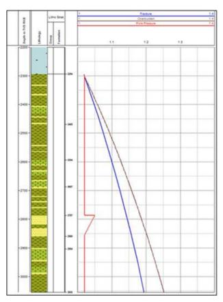
Figure 1. Example of a Pore Pressure, Fracture Gradient Chart
