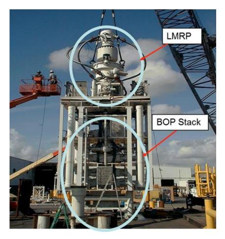
Figure 6a. Photo of a Typical Subsea BOP Stack
