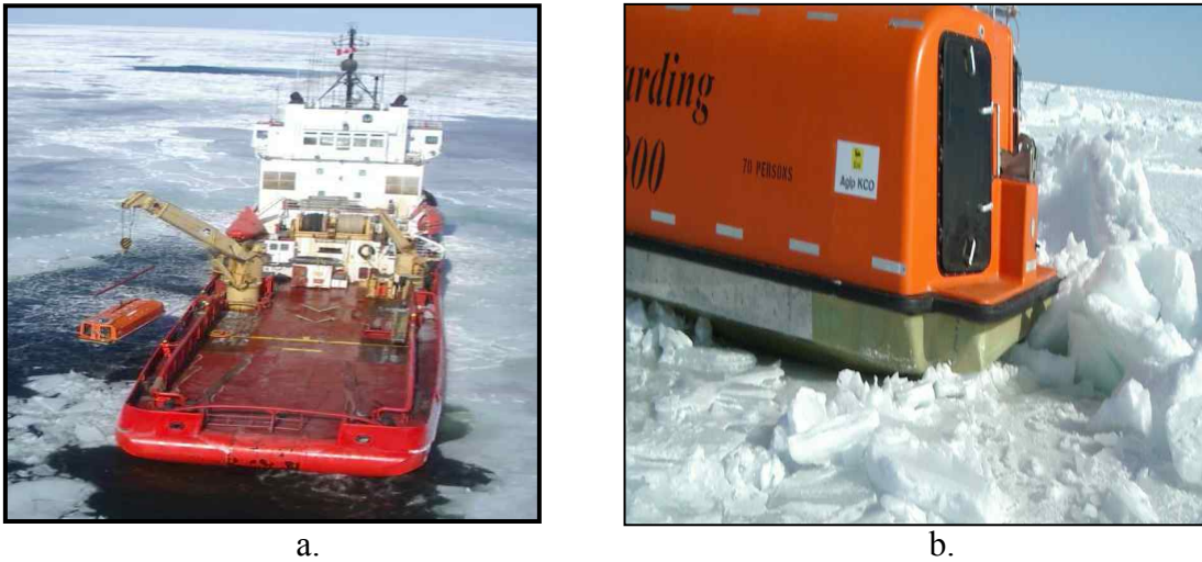
Figure 10. Lifeboat hull-ice interaction study (a) craft deployment and recovery icebreaker and (b) lifeboat. (Photos: Fleet Technologies)
