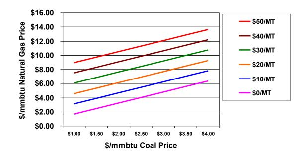
Figure 11. CO<sub>2</sub> Price Impact on Coal to Natural Gas Switching in Currently Operating Power Plants
