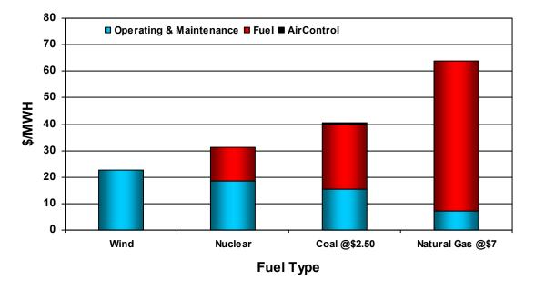
Figure 14. Variable Costs for Power Generation by Fuel Type<sup>42</sup>
