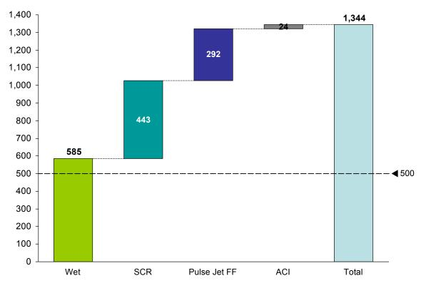
Figure 4. Estimated Capital Cost for Environmental Upgrades (\$/kW) to a 300 MW Coal Plant<sup>12</sup>
