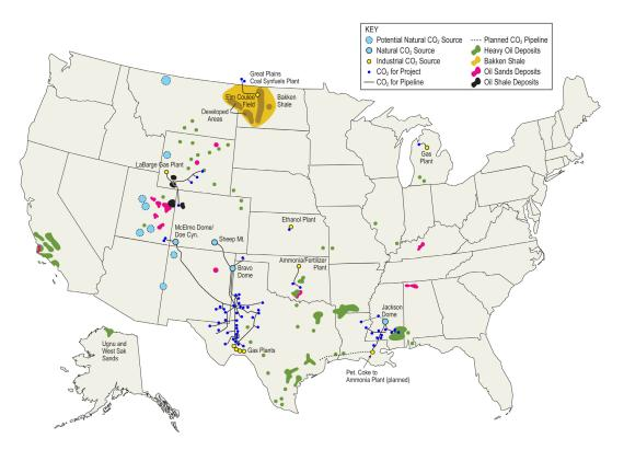
Figure 3. The current carbon dioxide EOR infrastructure, areas of development, and domestic oil resources in unconventional reservoirs, including the fractured Bakken shale of the Williston Basin. Source: DOE, National Energy Technology Laboratory, *Unconventional Fossil Energy Resource Program, Program Fact Sheet*, April 2011, www.netl.doe.gov/publications/factsheets/program/Prog100.pdf.
