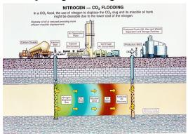
Figure 2: Illustration of the concept of EOR, where gas is pumped into the reservoir forcing oil to the production well. Source: DOE, NETL, at http://www.netl.doe.gov/technologies/oilgas/EP\_Technologies/ExplorationTechnologies/eordraw.html
