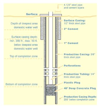
Figure 2. Example of a gas well (diagram is not to scale and has been dramatically shortened).<sup>35</sup>
