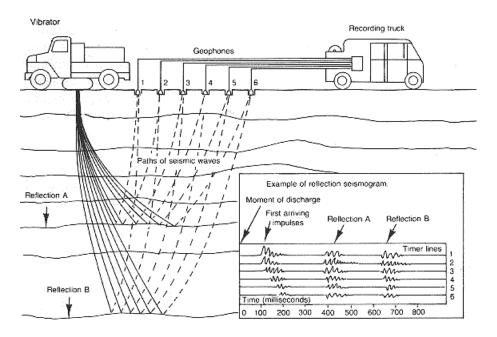
Figure 1. Seismic survey using a vibrator truck. Source: Heavy Oil Science Centre, Seismic Operations: A Backgrounder
