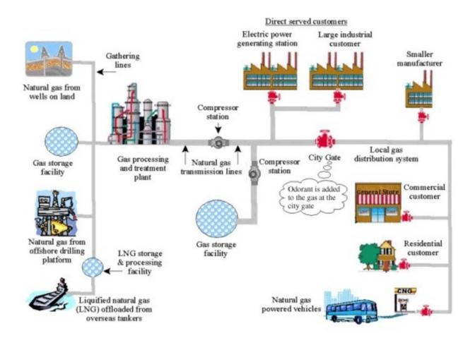
Figure 1. Schematic of a Typical Natural Gas Pipeline System (PHMSA, 2010a)
