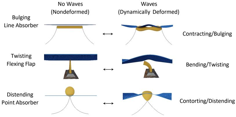
Three flexWEC archetypes - illustrating their methods of operation: ocean waves induce active deformations into the wave energy converter structures. The structures are made from distributed embedded energy converters (DEECs) that can convert those dynamic deformations directly into electricity; ocean wave energy conversion occurs throughout the structure without need to concentrate loads into a singular prime-mover or lone generator.
