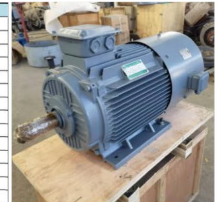
Rated 500rpm 20kW Generator (In transit)
