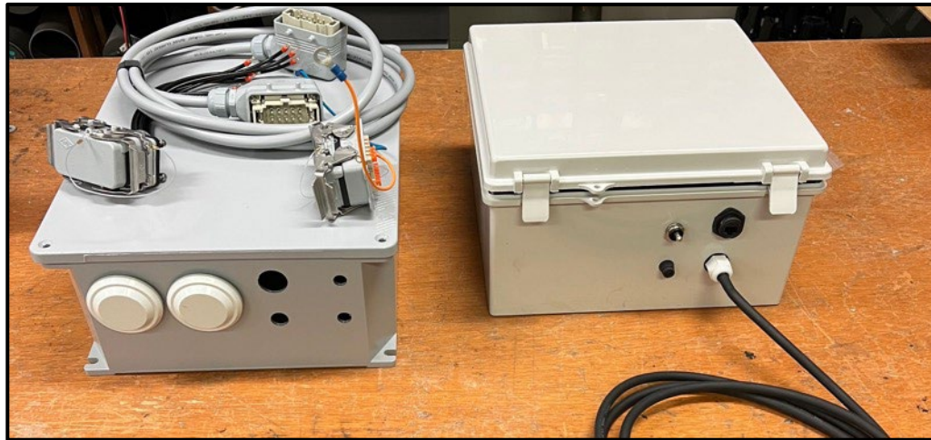
Left; SkyCharge Wireless Charging Pad Electronics Box, Right; FAU repackaged Electronics Box
