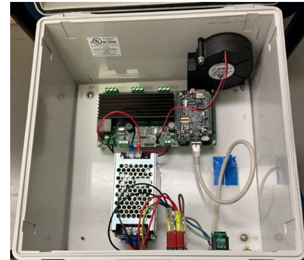
Inside view of FAU repackaged Electronics Box
