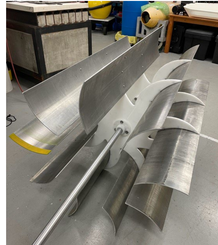
Fabricated and Assembled: 9 blade USWW
