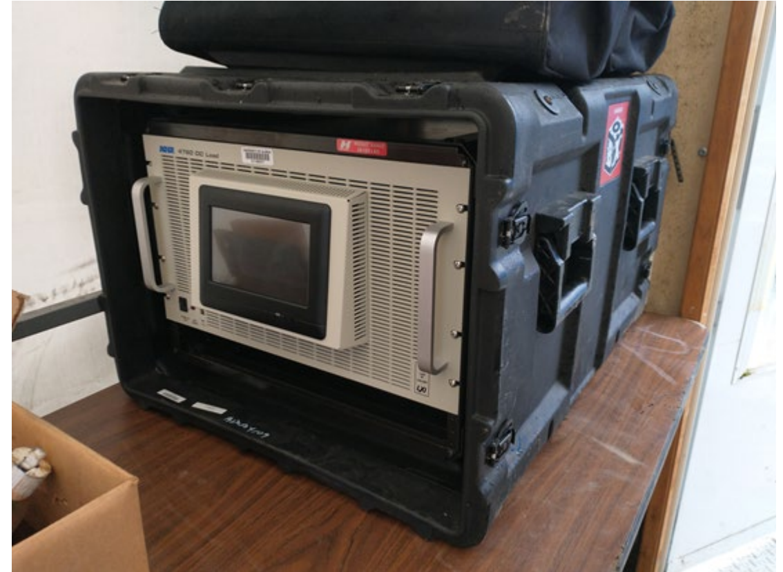
6 kW DC Load Bank used during Water Horse (WPTO) and SHARKS (ARPA-E) testing in 2021
