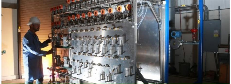
An engineer monitors a feed control system for a new, energy efficient pilot process for producing ethylene, one of the most energy-intensive and commonly manufactured chemicals.
