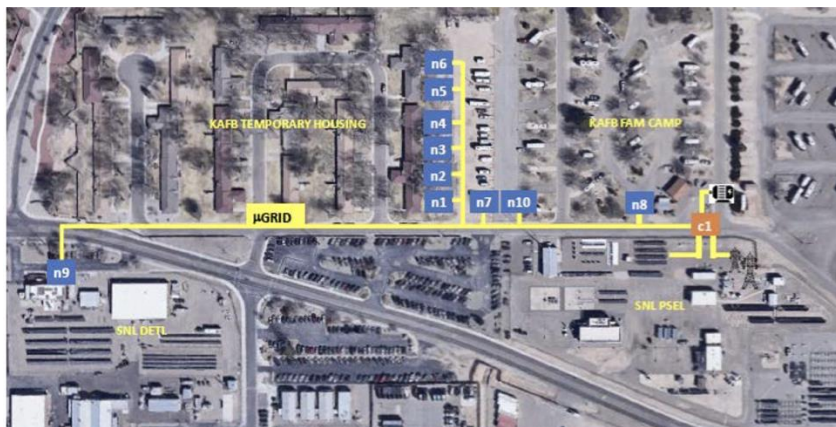
Figure 6 - Installed and operational DC/AC hybrid microgrid on Kirtland AFB. This Sandia/Emera project has been operational since December 2019
