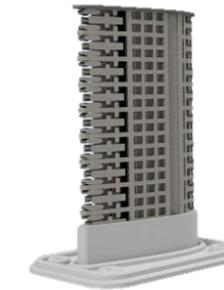
External Surface Removed in CAD
