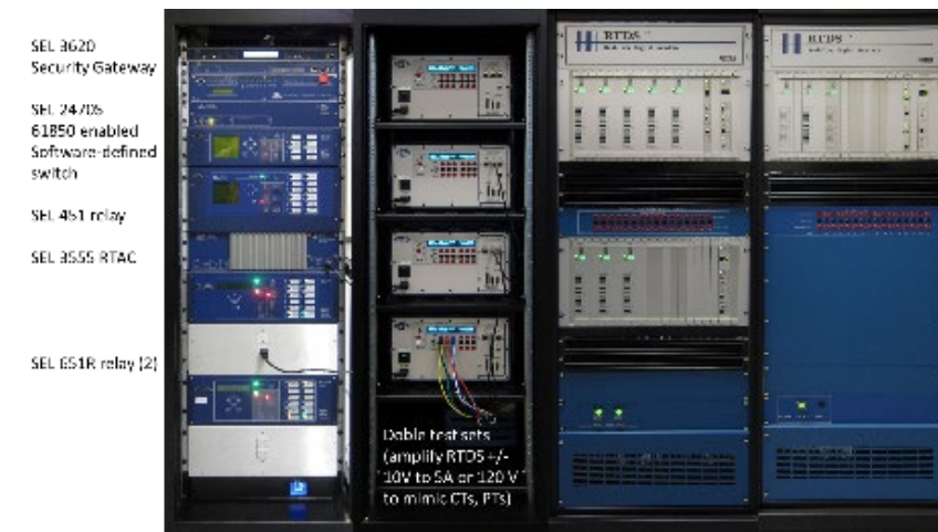
Real-Time Distributed Control system used for initial controller demonstration
