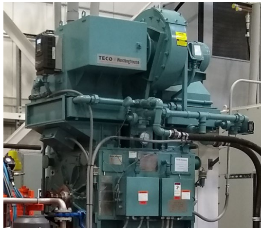
Prototype 1 MW, 15,000 RPM Induction Machine
