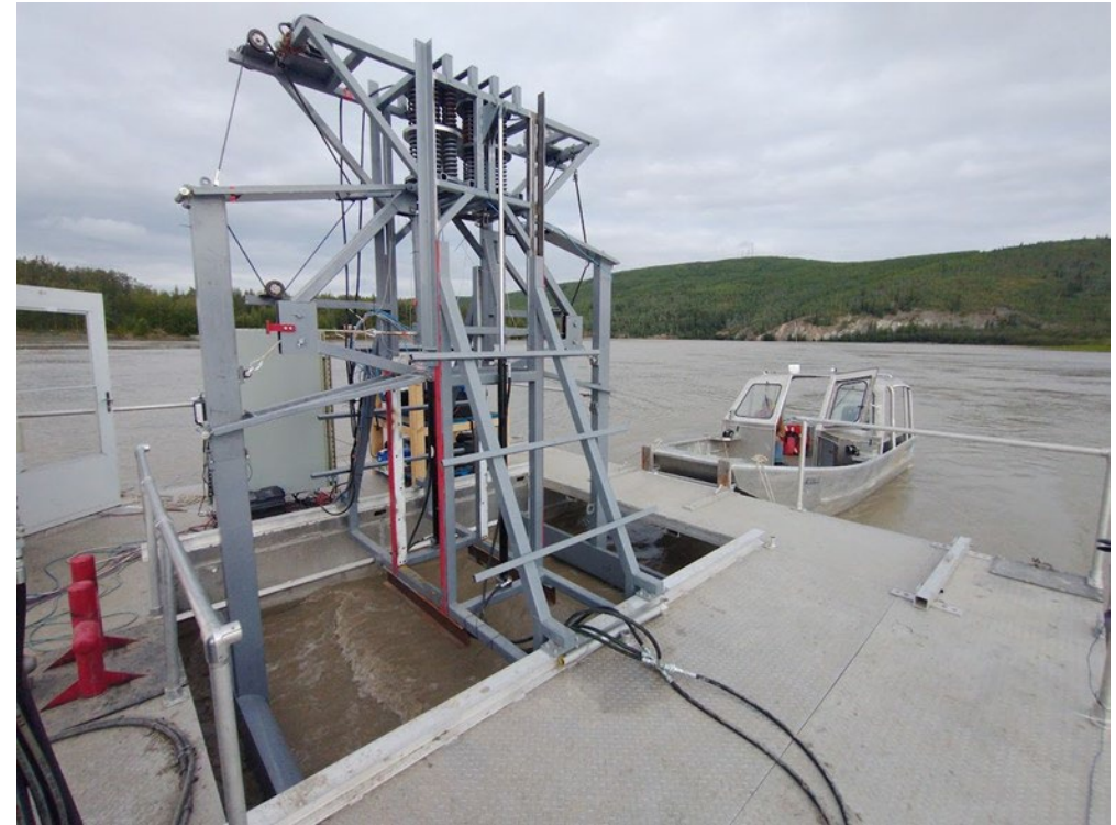
2021 Prototype – dual oscillators through barge moonpool
