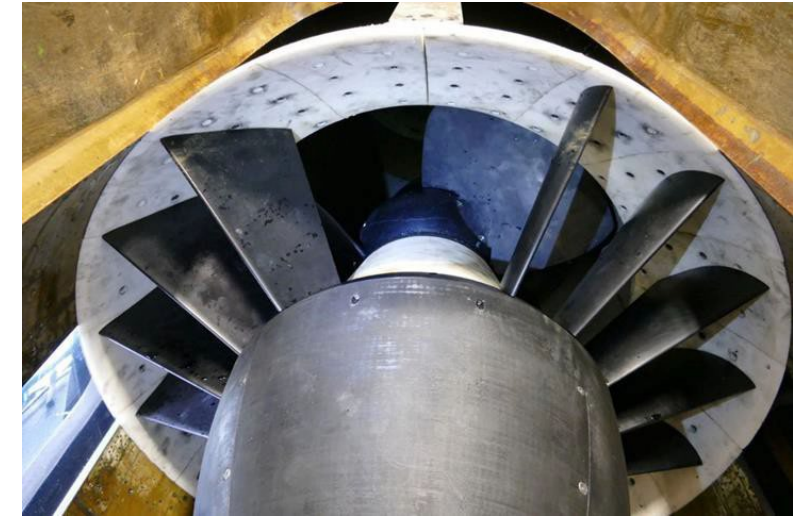
IGV blades removed to simulate a fault condition
