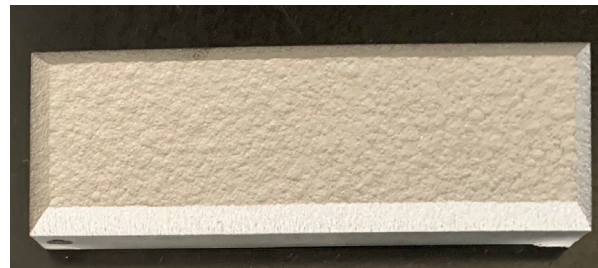
Typical Cold Spray Deposit (Top View)
