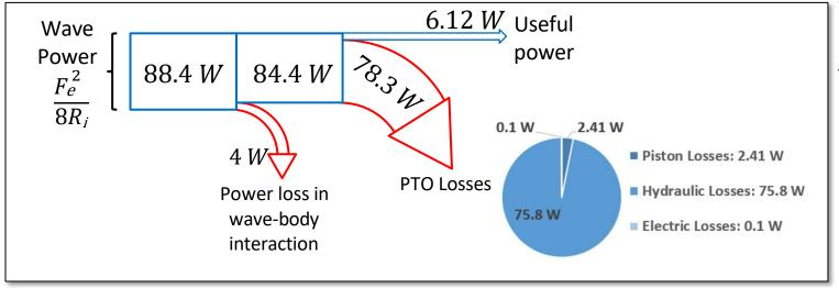
WEC PTO co-optimization in practice Numerical optimization of a novel power take-off design in parallel with control design
