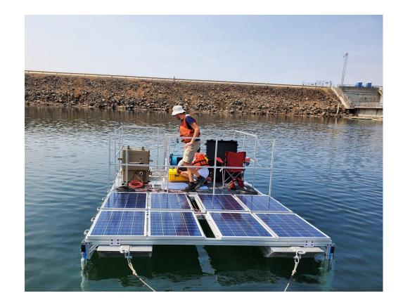
• Two versions of the mobile platform (ROV) were implemented to handle differences in flow. This allows the platform that is best suited for the specific flow conditions to be selected and demonstrates the flexibility of the system.
