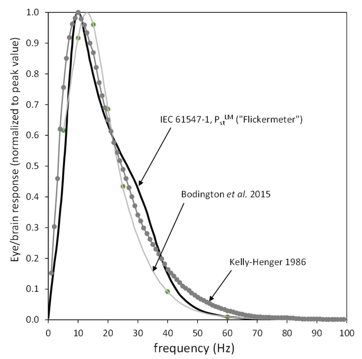
Figure 8. Sensitivity curves for direct flicker, one by Kelly-Henger (1986), one by Bodington et al. (2015), and one for the IEC's "Flickermeter" measure (De Lange 1961). Plot after Garner 2020.
