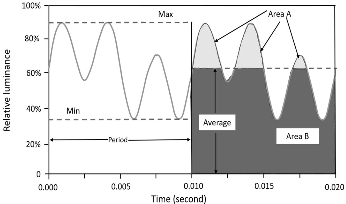
Figure 5. A periodic TLM waveform illustrating period, frequency, and values critical for calculating percent flicker and flicker index.
