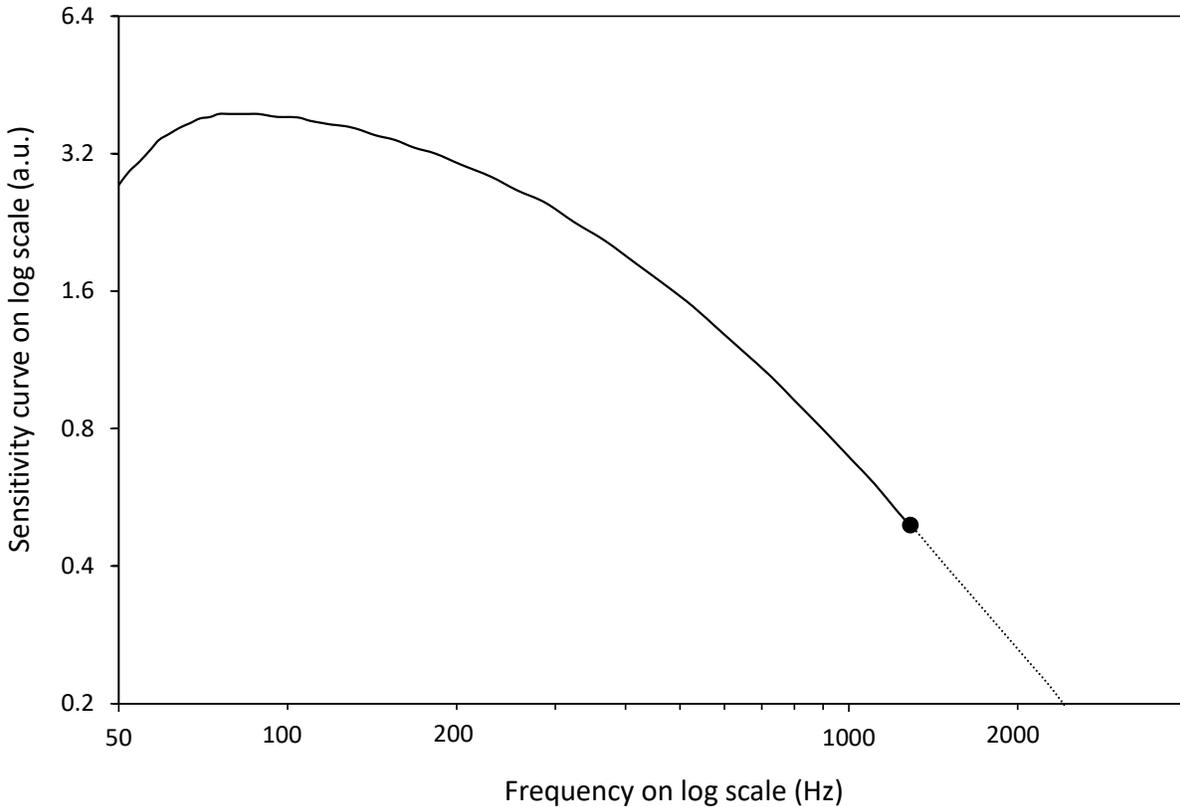
**Figure 9. Sensitivity curve for sine waves at different frequencies, used to normalize the Fourier frequency amplitudes in the SVM calculation, plotted on log scales. The black dot indicates the highest frequency at which there was a datapoint. Plot after CIE 2016.**
