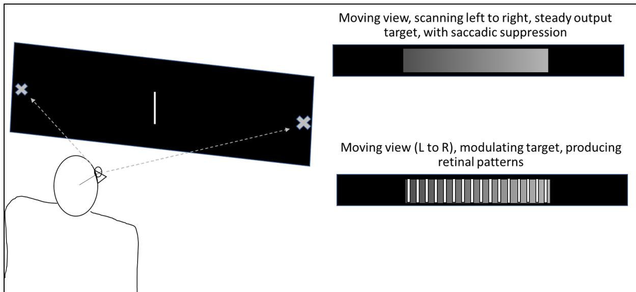
**Figure 10. An illustration of the phantom array effect resulting from a saccade across a vertical target with either steady or modulating luminance. The repeated pattern from the modulating target is visible because of the target's high contrast and because the pattern on the retina is close to maximum contrast sensitivity.**
