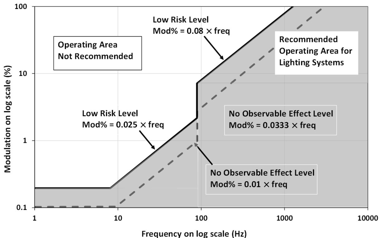
Figure 11. IEEE 1789-2015 recommended operating area to reduce visual discomfort, annoyance, and health effects of modulating light. Combinations of Percent Flicker (Modulation (%)) and fundamental frequency at the Low-Risk and No Observable Effects Levels fall in the shaded area. (Figure adapted from IEEE 1789-2015.)
