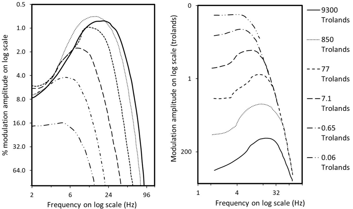
**Figure 7. Temporal contrast sensitivity curve derived from Kelly (1961) showing direct flicker thresholds for a large visual field at different retinal illuminances. The modulation is expressed as percentage modulation in the left plot and absolute modulation in the right plot (after Boyce 2014 and Kelly 1961).**
