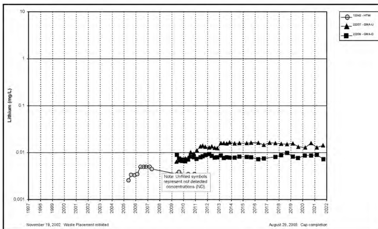
Figure A.5.5-10. Cell 5 Lithium Concentration Versus Time Plot for HTW, GMA-U Well, and GMA-D Well
