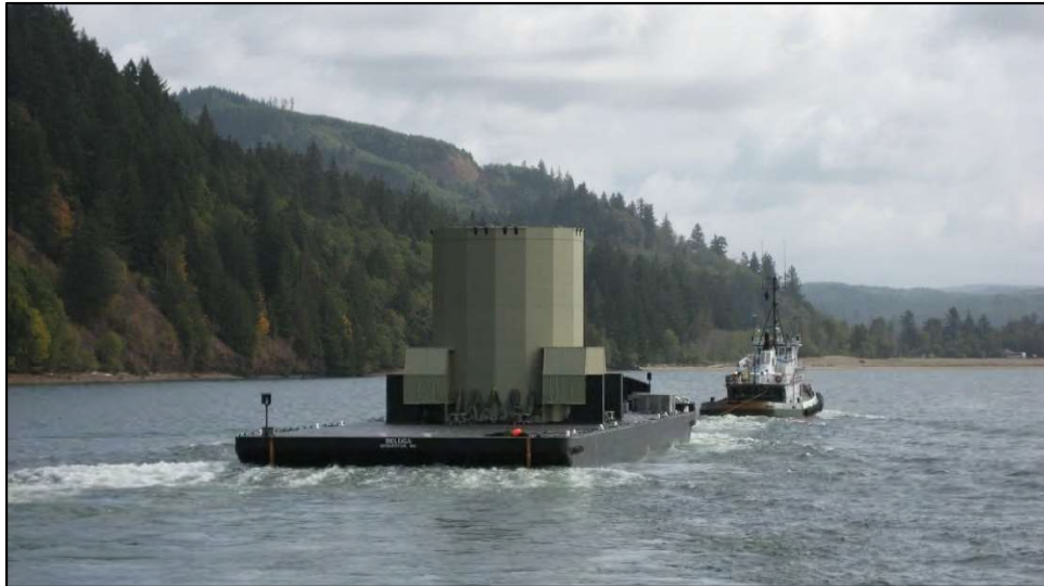
Figure 2-11: Example of Transport Barge with Cruiser Reactor Compartment Package
