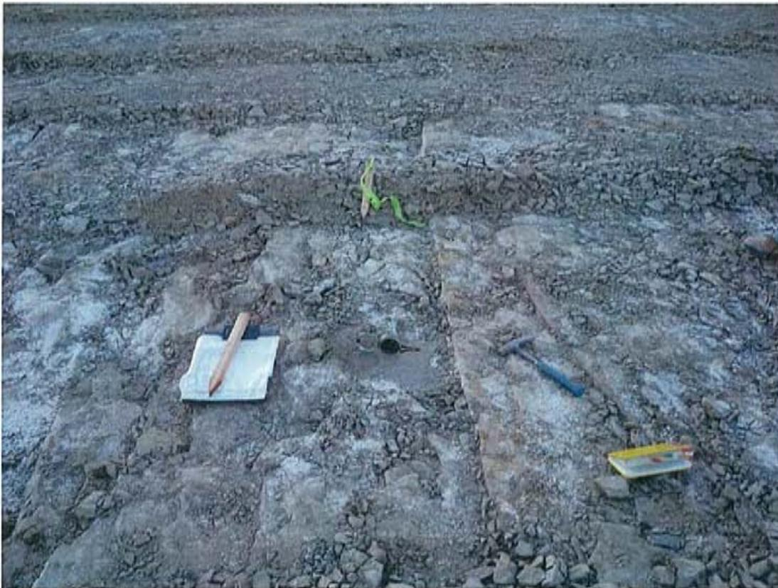
*Figure 17. West-Striking Vertical Joint System Spaced about 1 to 2 Ft Apart with Gypsum Coatings at Location 11 of November 24*
