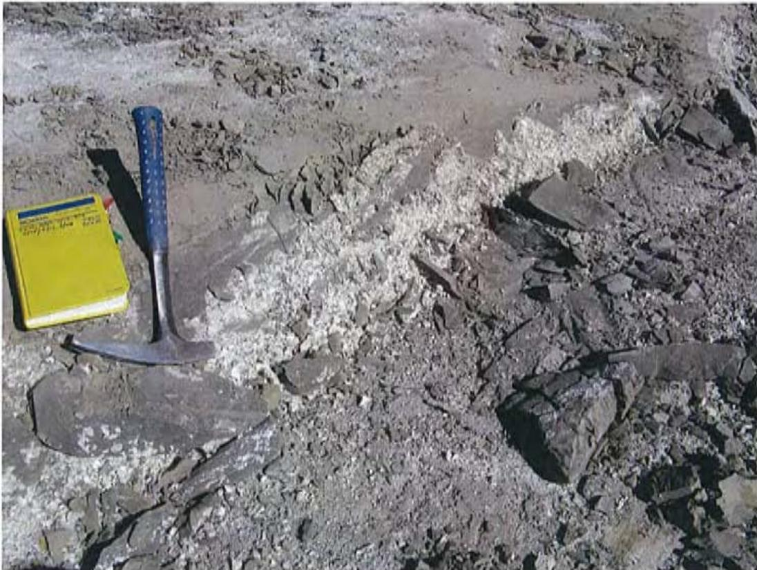
*Figure 6. Abundant White Gypsum (Satin Spar) Along Joints and Bedding Surfaces in Weathered Mancos Shale on Excavation Floor*
