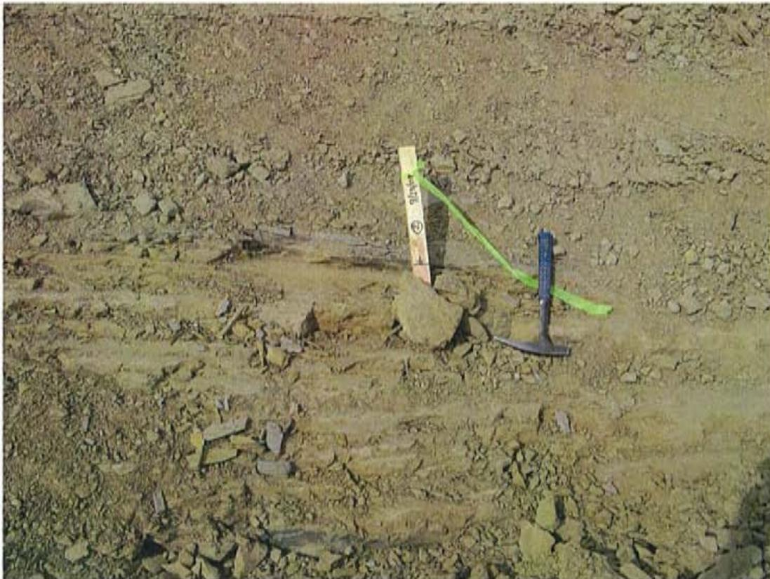
Figure 9. Very Fine Grained Limonitic Sandstone Bed About 6 Inches Thick Near Center of North Side Slope of Excavation
