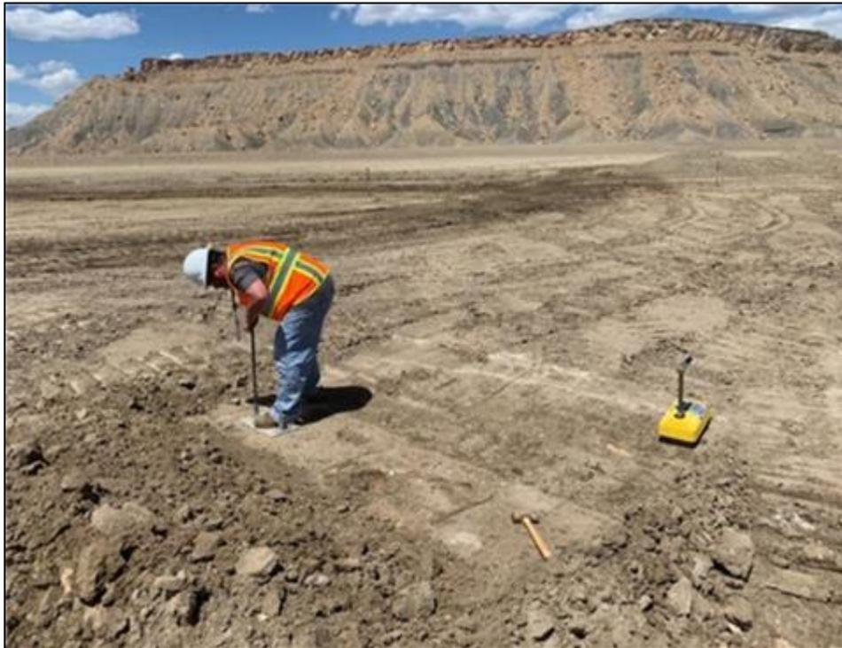
*Photo 19. Moisture/Density Testing May 2020*
