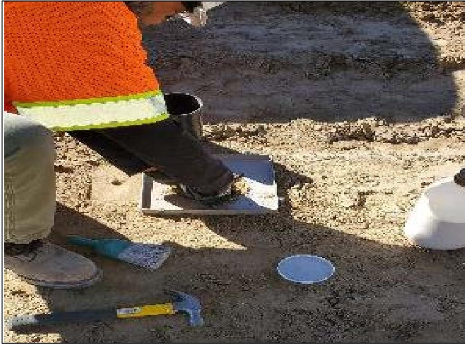
*Photo 37. QC Performing Sand Cone Test September 2020*
