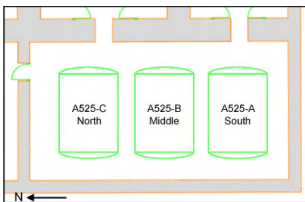
Figure 8-6. 10,000-Gallon Storage Tank Area, 309-Foot Level
