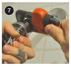
Ensure that connections will not leak while preventing damage by using buffer material.
