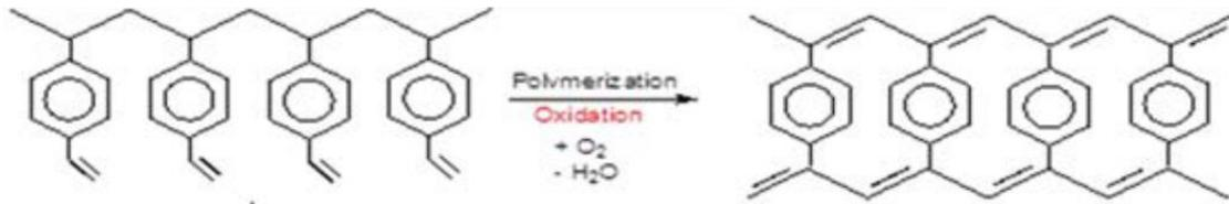
Synthesis and carbonization of triethylammonium-based poly(p-phenylenevinylene) (PPV) [Universitat Stuttgart; Michael R. Buchmeiser]
