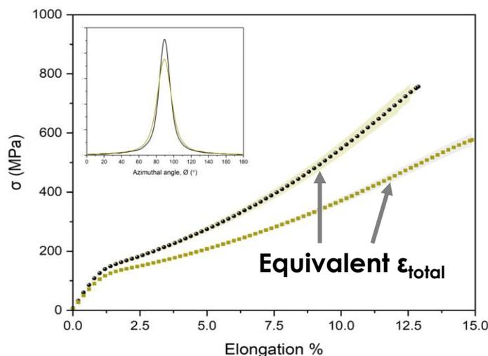
Precursor fiber conditioning can enable a wider range of fiber quality to achieve high performance CF
