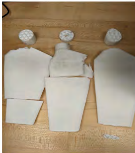
Figure 7. Blade Failures at the Root
