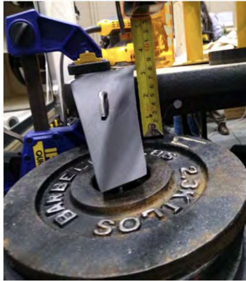
Figure 5: Point of failure at 20 lbf (88N) during blade deflection testing.
