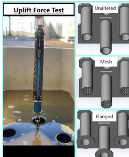
Figure 15: Uplift force test and three pile types.
