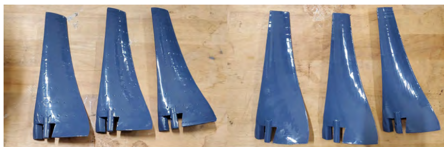
Figure 5. Final blade prototypes: with dimples (left three) and without dimples (right three)
