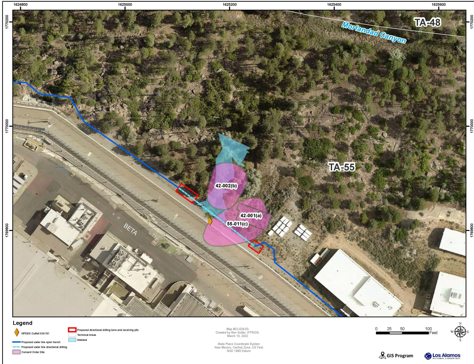
Figure 4. Detail of the proposed water line route, the TA-55 wetland, and proposed directional drilling elements.
