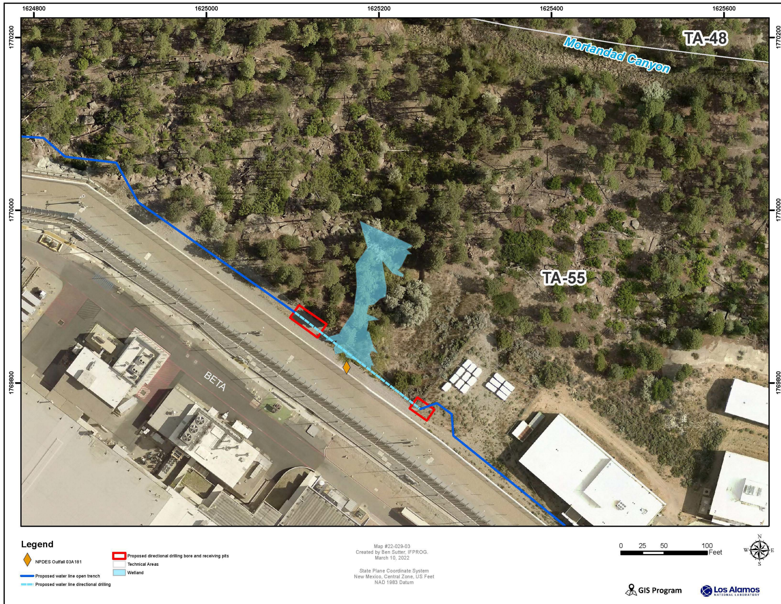
Figure 4. Detail of the proposed water line route, the TA-55 wetland, and the proposed directional drilling elements.
