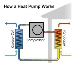
Outdoor coil absorbs heat from the air, then the compressor concentrates the heat, and finally the indoor coil releases heat into the air.
