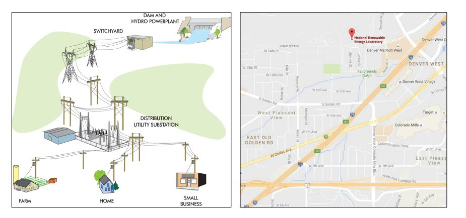
The high voltage transmission system is like our interstate highway system, while The distribution system is like our city streets.
