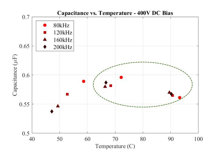
In capacitors,  $|Z| = 1/(2\pi fC)$ , so operating regions in which *capacitance decreases with temperature are advantageous* for performance and reliability.
