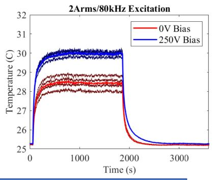
Individual device characterization looks favorable for DC Link applications: High ripple current capability, Stable capacitance w/ DC Bias, Low loss at high temperature.
