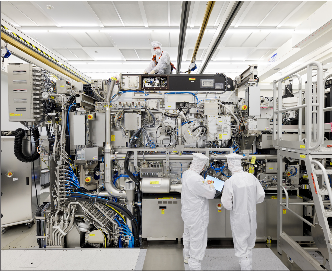
The EUV Lithography system, shown here as a commercialized product, was created by a highly unusual collaboration between industry partners and the Federal government.
