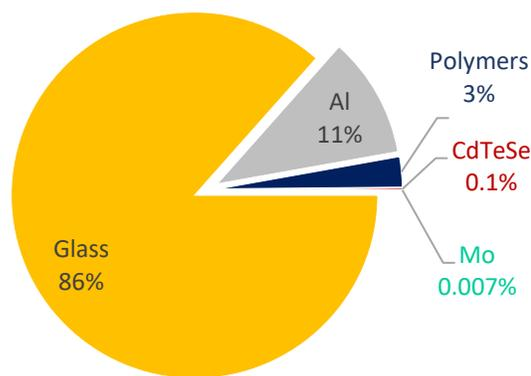
Figure 6. Materials breakdown by mass for a CdTe module.
