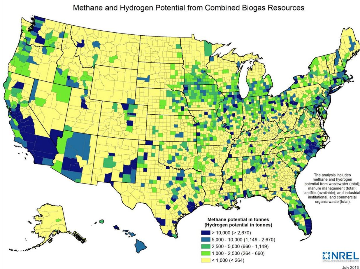
**Figure 20. Methane resource potential from combined biogas sources in the United States by county**
