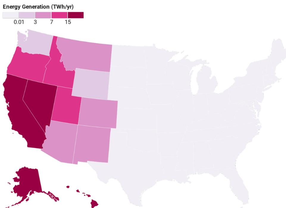
Figure 30. Annual energy production technical potential for hydrothermal geothermal energy
