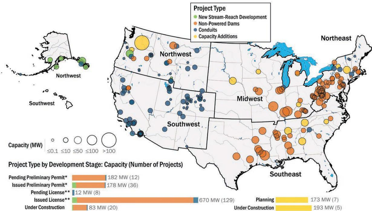
Figure 37. Hydropower project development pipeline by project type, region, size, and development stage as of the end of 2019
