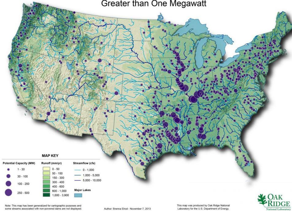
Figure 34. Map of U.S. non-powered dams with potential capacity greater than 1 MW
