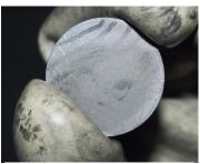
A small disk of plutonium metal at TA-55.
