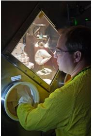
Glovebox work in the TA-55 machining area.
