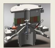
Cutaway Diagram – Z Beamlet Transport Tube
