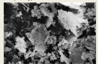
Scanning electron micrograph of microstructure in porous magnesium oxide
