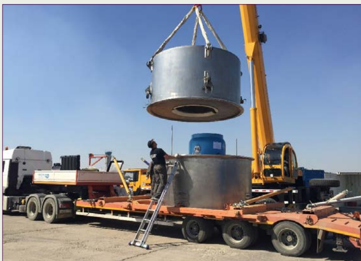
The SKODA VPVR/M spent fuel shipment cask is enclosed in a TUK-145/C over-package, which is licensed for air transport and protects its contents from extreme shocks.
