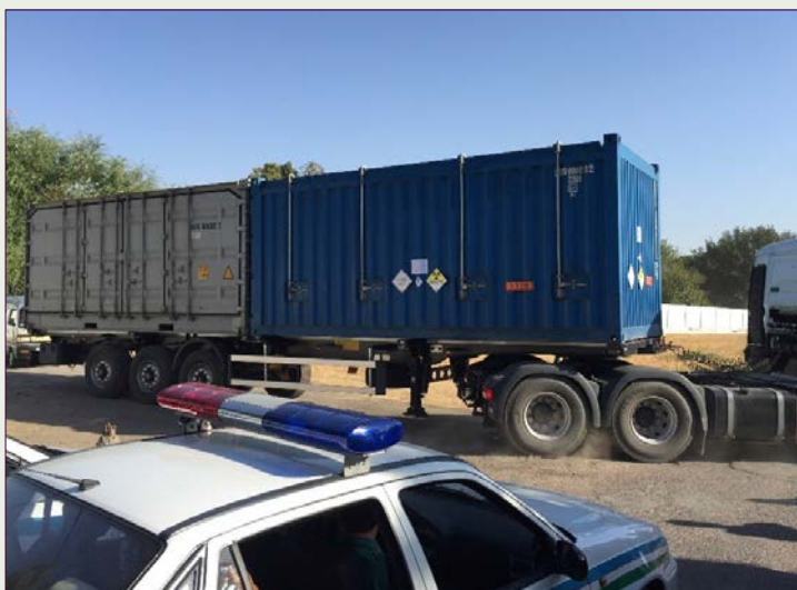
An ISO transport container carrying the SKODA VPVR/M spent fuel shipment cask travels from the Foton reactor facility to Tashkent International Airport under police escort.
