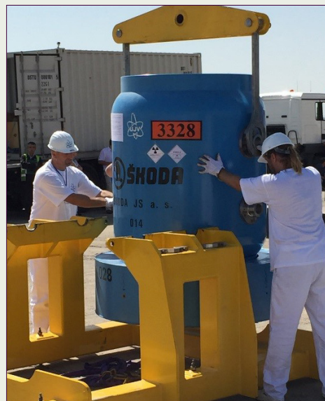
The SKODA spent fuel shipment cask is prepared for transfer to its TUK-145/C over-package at Tashkent International Airport.
