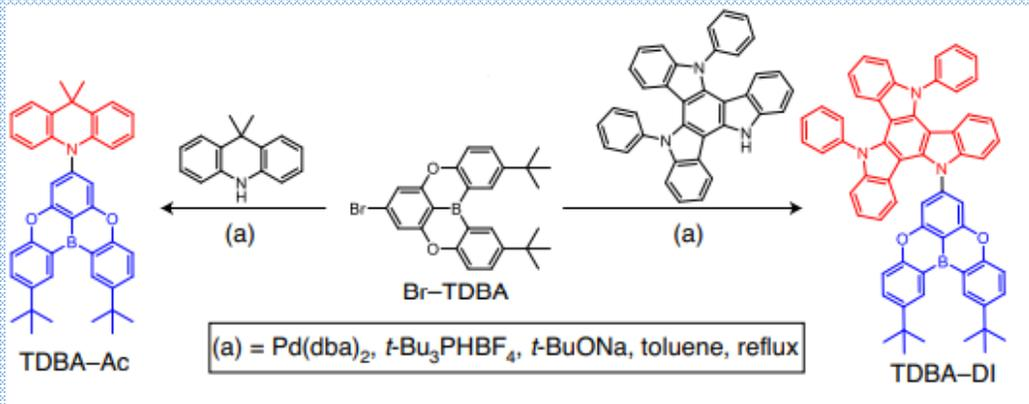
These OLEDs are based on TADF emitters bearing symmetrical and rigid oxygen-bridged boron acceptors
