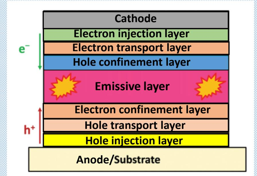
*The lifetime of blue OLEDs is severely affected by excited host molecules instability. Efficient, quick energy transfer from the host to the guest emitter before the host molecules' degradation is expected to suppress the formation of the exciton quenchers and non-luminescent species.*
