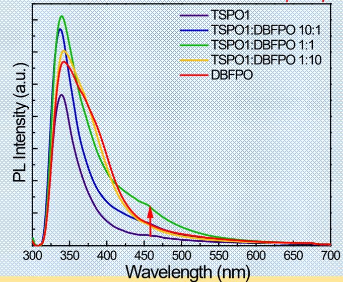
Design rule: singlet and triplet levels ( $S_1/T_1$ ) energy levels of the exciplex to be higher or equal to those of the blue emitter to prevent back-energy transfer from the latter to the exciplex.
