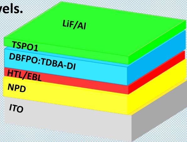
*These devices exhibited identical emission color ( $\lambda_{max}=458$  nm) and below bandgap  $V_{ON} = 2.5$  V electroluminescence.*
