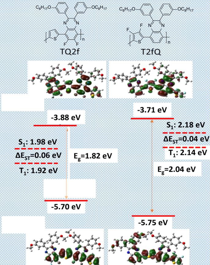
The replacement of the F atoms from the quinoxaline to the thiophene had significant effect on the **energy levels** along with the **dihedral angle** between the two adjusted building blocks.
