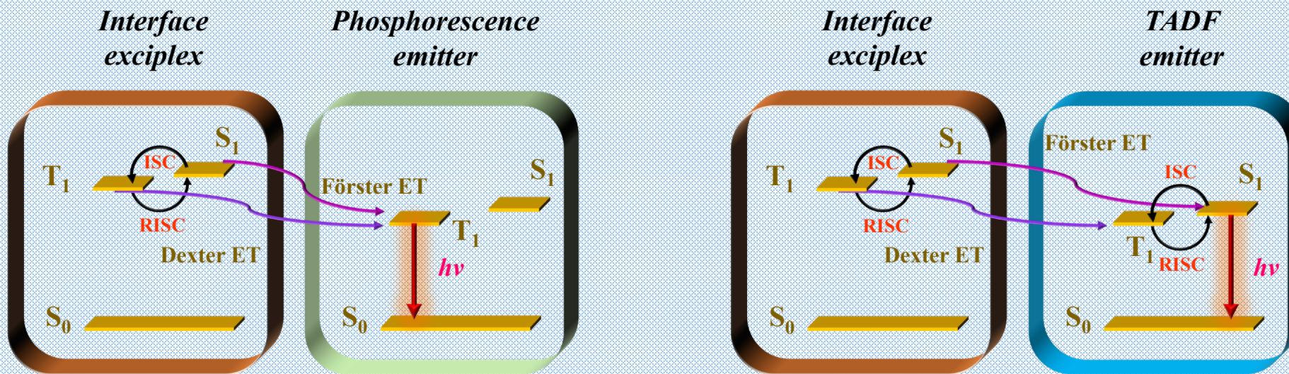
*OLEDs based on interface exciton hosts show low driving voltages, reduced efficiency roll-off, high power efficiencies and satisfied device lifetime.*
