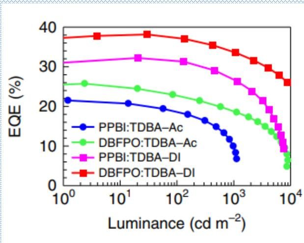
Significant efficiency roll-off and short device half-lifetime ( $T_{50}$ ) of less than 2h at  $500 \text{ cd m}^{-2}$ .
