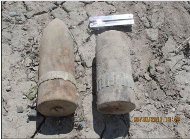
3-in inert proofing projectiles
